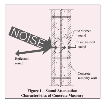
noise over a wide range of frequencies; and it can be an effective sound absorption material for absorbing noise generated within a room. This TEK discusses the sound absorption and sound transmission properties of concrete masonry, and provides general design guidance to help provide a good acoustic environment.
