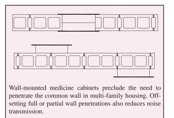
Figure 7—Minimize Wall Penetrations
