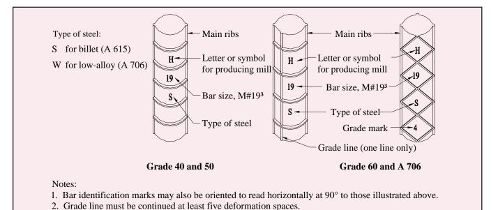
Figure 1—ASTM Standard Bar Identification Marks (ref. 14)
